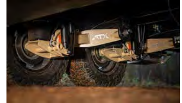
Tough Airbag Suspension CruiseMaster ATX 4.5T Level 4 Airbag + Bosch ABS. Australian Made suspension, full off road capable.
