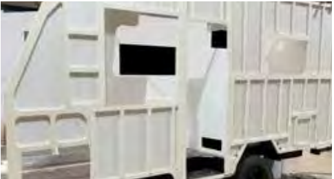
Polyresin Composite walls. Wall framing / inner skin is constructed of a polyresin composite. PRC is a water and humidity resistant product which will withstand Australia's varied weather conditions
